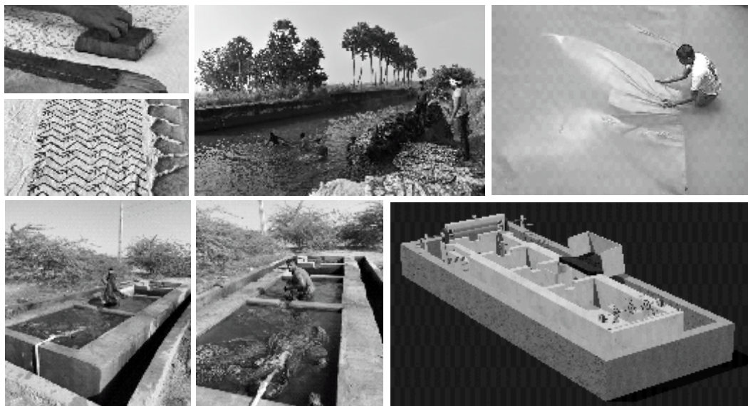
Figure 1. a. Printing with mordants; b and c. Washing at river canal d and e. Washing in tanks; f. 3D model of the proposed tank system
