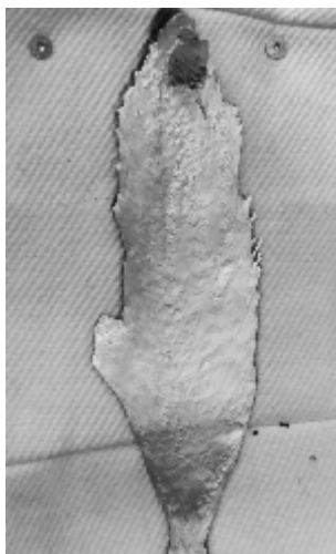
Figure 1: Sticking of molten aluminium on para-aramid fabric
